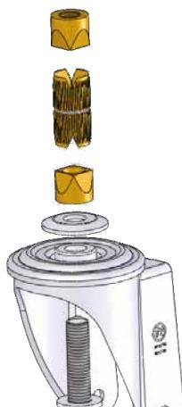
We recommend fastening the castor with expansion stem to the tubular structures by using adequate tightening torques. Insufficient tightening torques can jeopardise the overall carrying capacity and/or the stability of the product.
