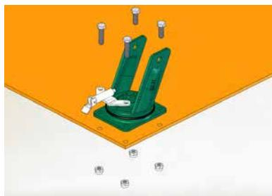
3. The bolt has to protrude through the nut by at least 3 threads.
