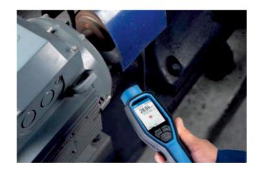
Enclosed parts for contact measurement
