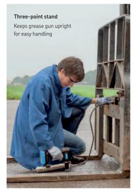
The tool's display indicates battery charge level, amount of grease dispensed, pump/motor speed and blocked lubrication points. This versatile grease gun provides two flow rates – low and high – and can dispense up to 15 grease cartridges per battery charge. The TLGB 20 can deliver pressures up to 700 bar (10 000 psi) and features a built-in light to illuminate the work area.
