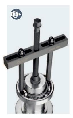
Removes bearing without dismantling machinery
