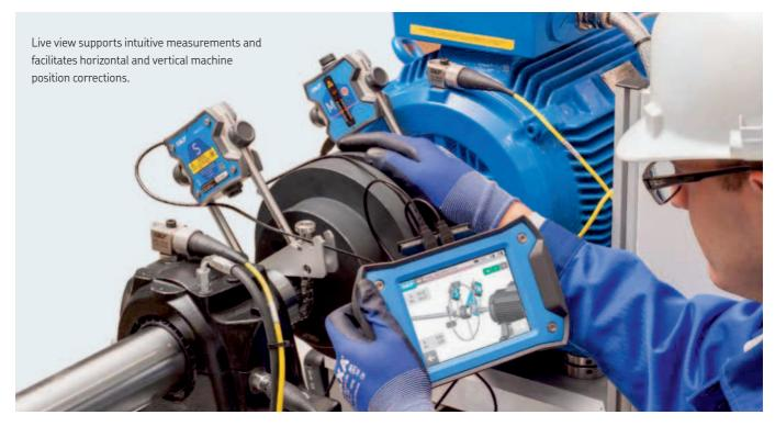
The advanced laser shaft alignment system with enhanced measuring and reporting capabilities
