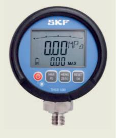
The Digital oil pressure gauge, THGD 100, is used to accurately measure the hydraulic pressure when mounting bearings using the SKF Drive-up Method.
