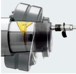
Poor bearing mounting techniques can significantly reduce the bearing service life.
