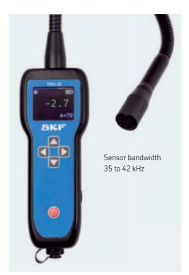
The TKSU 10 helps users to easily find leaks from a distance, even in noisy industrial environments, via its ultrasound measurement sensor. The built-in LED display assists the user in adjusting sensitivity and shows the measured ultrasound noise from leaking air, allowing the quantification of leaks and prioritization of repairs.
