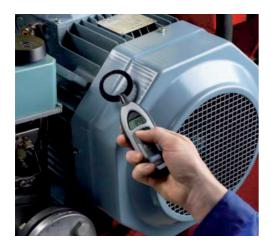
Electric motors are more vulnerable to suffer electrical erosion in bearings when controlled by a Variable Frequency Drive. When incorporated into a predictive maintenance programme, the EDD Pen can help detect bearings more susceptible to failure, and to a significant degree, prevent unplanned machine downtime.
