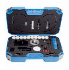
Portable grease analysis kit for field use
